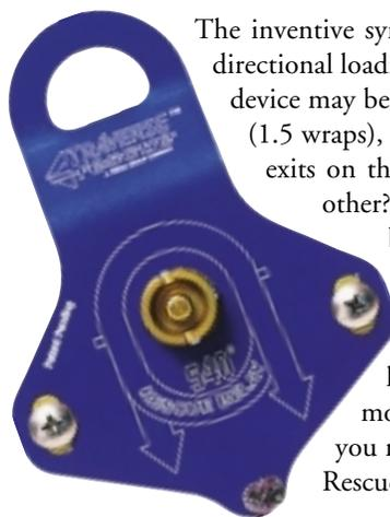
The inventive symmetrical design of the 540°™ Rescue Belay allows bi-directional loading and locking, and thus either end of the rope exiting the device may be used as the load line. You will have noticed that it is 540° (1.5 wraps), not 360° (a full circle), so the rope begins on one side and exits on the other, or was that exits on one side and begins on the other? It doesn't matter; since it's bi-directional, either side can be the end or the beginning.
